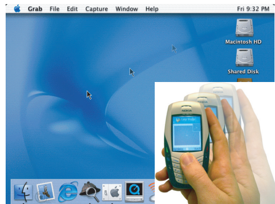
Figure 3: The sweep technique can be used to control a cursor by waving the phone in the air.
