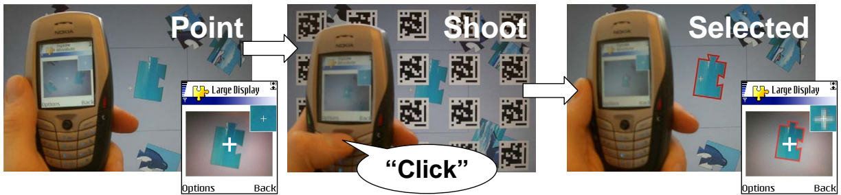
Figure 2: Point & shoot interaction: The left screenshot shows the phone screen as the user is aiming at the highlighted target. The cursor on the phone is active and the locus of attention and the cursor on the display is inactive. Pushing the joystick to the left indicates a selection at the location of the cursor on the phone display. Then the visual code grid is briefly displayed for computing the target coordinates as shown in the middle screenshot. The grid disappears again and a mouse selection occurs in the target region.
