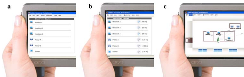
Fig. 7 The three interfaces implemented on an OQO handheld for study of spatial references, from left to right: a alphabetical list, b spatial list, c iconic map
