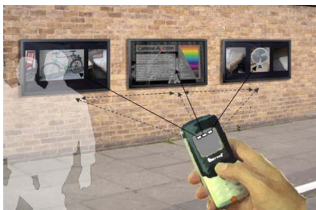
Fig. 1 The RELATE model for spatial interaction is based on relative positioning of potential target devices near a mobile user, and provision of corresponding spatial references in the user’s device
