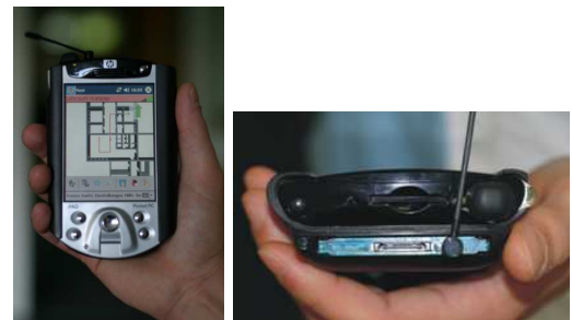
Figure 1: iPAQ PDA running the ABP localization system and with attached RFID reader.
