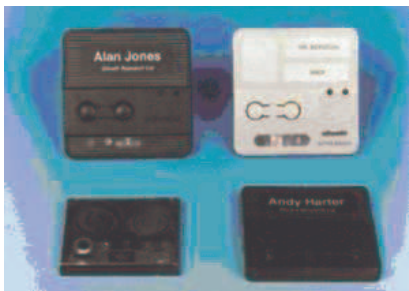
Figure 3 Four generations of active badges
