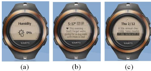
Figure 7: Suunto n3 wriststop computer with Microsoft’s MSN ® Direct Service. (a) up-to-date weather information, (b) received message, (c) Microsoft ® Outlook ® appointment, Source: [14]
