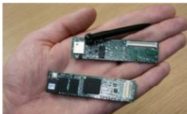
Each sensor contains a small embedded computer, shown (Image: Danny Hughes, University of Lancaster)
