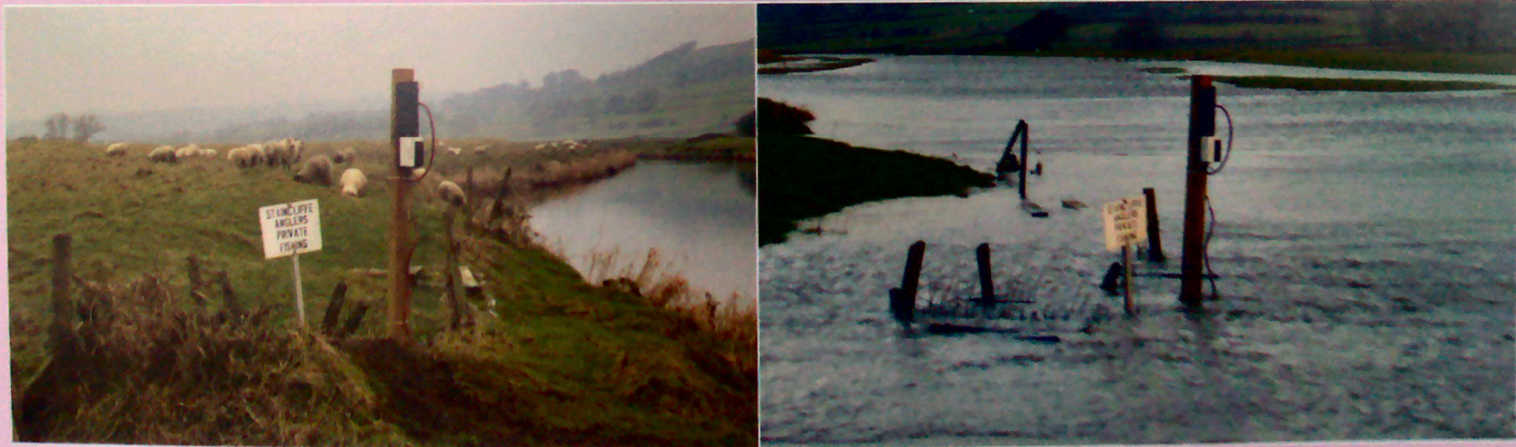
A depth monitoring sensor before and during a flood
